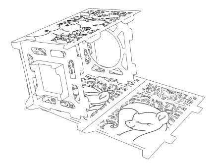
As the last panel is attached to the top and bottom frames, guide the tabs on the last panel into the slots on the first one. It may be helpful to partially seat all of the horizontal tabs before working on the panel tabs.
