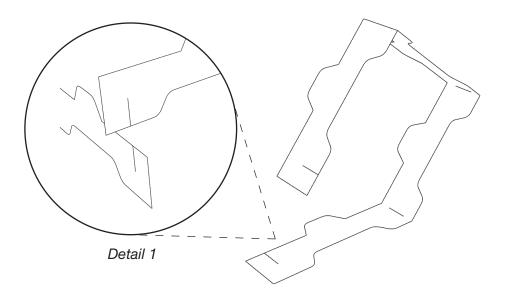
Attach the folded bottom support **D** into base frame **B**. Work one tab at a time, and carefully slide the tabs on the bottom support into the slots on the base frame. Bend the tabs down on the other side once they are fully seated.
