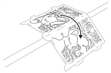
To bend, place the seam at the edge of a table with a sharp corner, and carfully apply pressure to the seam. Keep panels face-up (tabs on the left, slots on the right.)
